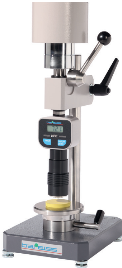
Test stand BS 61 II with HPE II and loading weight
